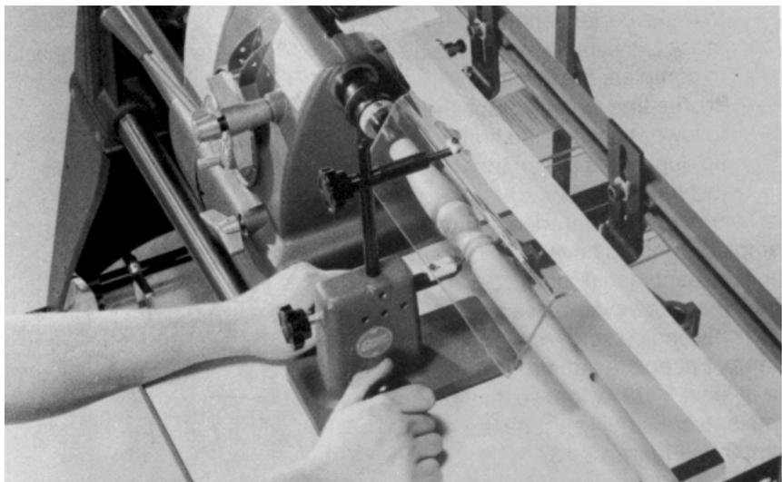
**Figure 13-10.** Spindles are duplicated from flat templates.
